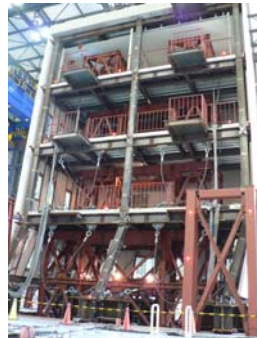
E-Defense Steel Collapse
